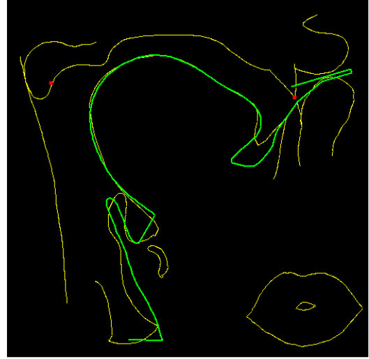
Figure 1: Fitting of the tongue model. A new speaker VT contours delineated by hand in yellow. Model contour in green. The larynx and the lip are also represented.
