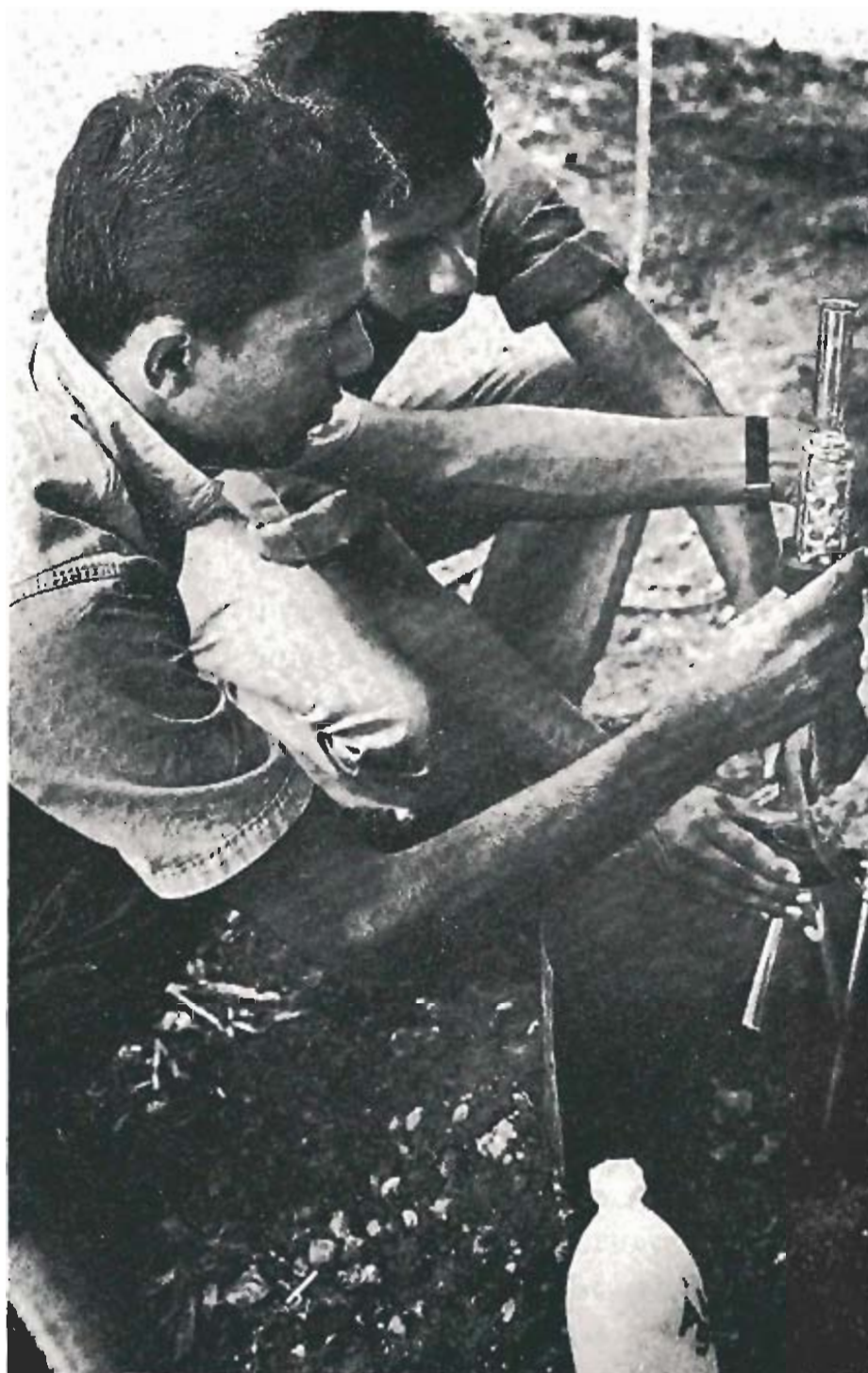
FIG. 3. Students of the University of Sri Lanka processing food samples in boiling alcohol, at the Polonnaruwa Field Station. Water for cooling the condenser is in a canvas water-carrier hanging above the apparatus.
