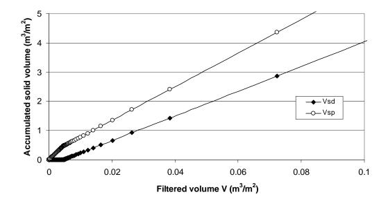
Fig. 7: Calculation of deposit specific resistance a as a function of filtered volume from the modelling and from the classical method for dead end filtration with the slope of the line t/V versus V.
