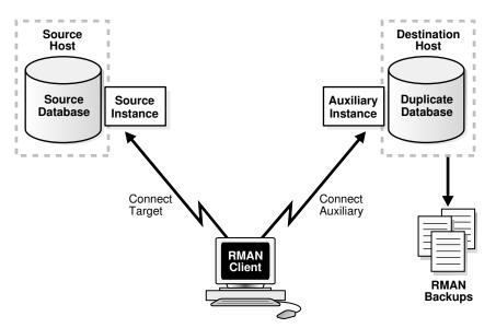
Figure 24-1 Backup-Based Duplication with a Target Connection
