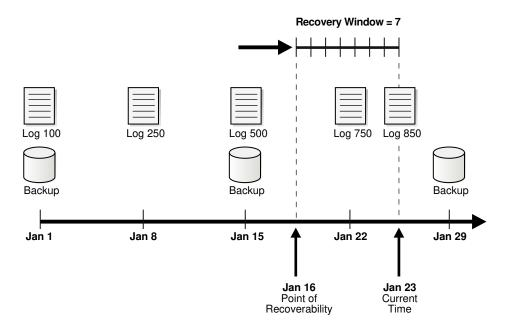
As illustrated in Figure 8-4, the current time is January 23 and the point of recoverability is January 16. Hence, the January 15 backup is needed for recovery, and so are the archived logs from log sequence 500 through 850. The logs before 500 and the January 1 backup are obsolete because they are not needed for recovery to a point within the window.
