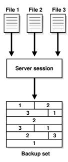
RMAN multiplexing is determined by several factors. For example, the FILESPERSET parameter of the BACKUP command determines how many data files to put in each backup set. The MAXOPENFILES parameter of ALLOCATE CHANNEL or CONFIGURE CHANNEL defines how many data files RMAN can read from simultaneously. The basic multiplexing algorithm is as follows:
