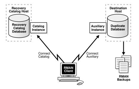
Figure 24-2 Backup-Based Duplication Without a Target Connection
