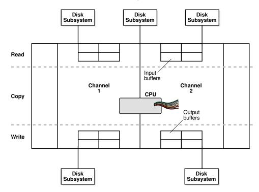
Figure 22-1 Phases of a Multichannel Backup to Disk
