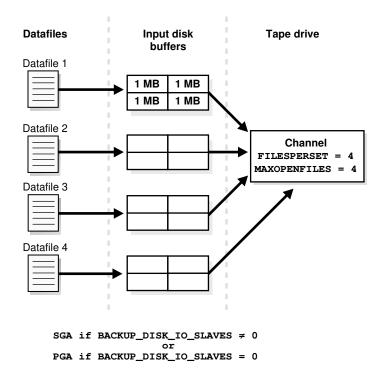
If a channel is backing up files stored in ASM, then the number of input disk buffers equals the number of physical disks in the ASM disk group only if the level of multiplexing is 1. For example, if a data file is stored in an ASM disk group that contains 16 physical disks, then the channel allocates 16 input buffers for the data file backup.
