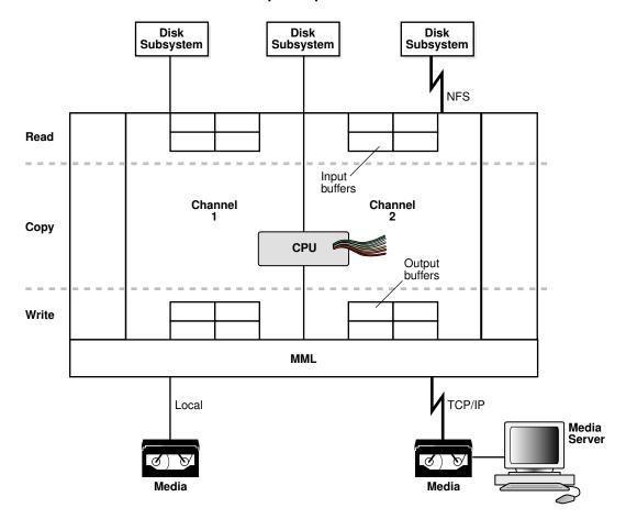
Figure 22-2 Phases of a Multichannel Backup to Tape
